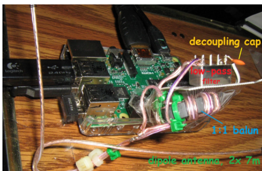
Figure 1 shows Joe's setup. Since the output generates a square wave, a low-pass filter is needed to filter out the high-frequency components. As you can see, the GPIO output is fed through a 0.1uF decoupling capacitor into a Mini-Circuits 10.7MHz low-pass filter, then to a 1:1 balun, which is connected directly to the
